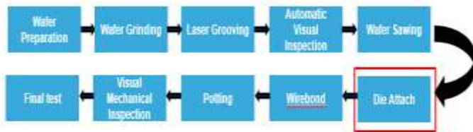
Fig. 1. Typical assembly process flow for tape and reel.
