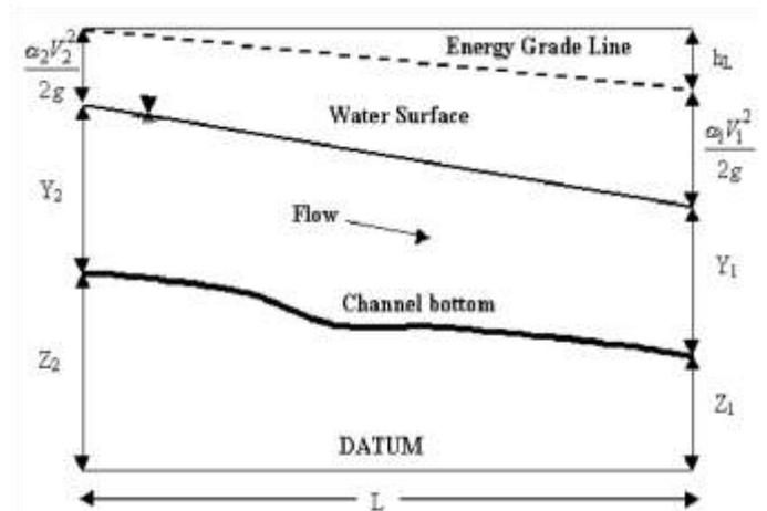
Figure 1. Depiction of energy equations in open channels (Istiarto, 2014)
