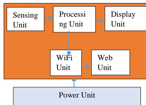
Fig. 1. The Block Diagram of Smart Waste-bin monitoring system
