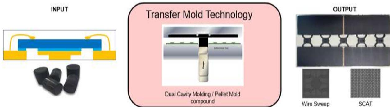
Fig. 3. Transfer molding process using pelletized molding compound on a dual cavity.
