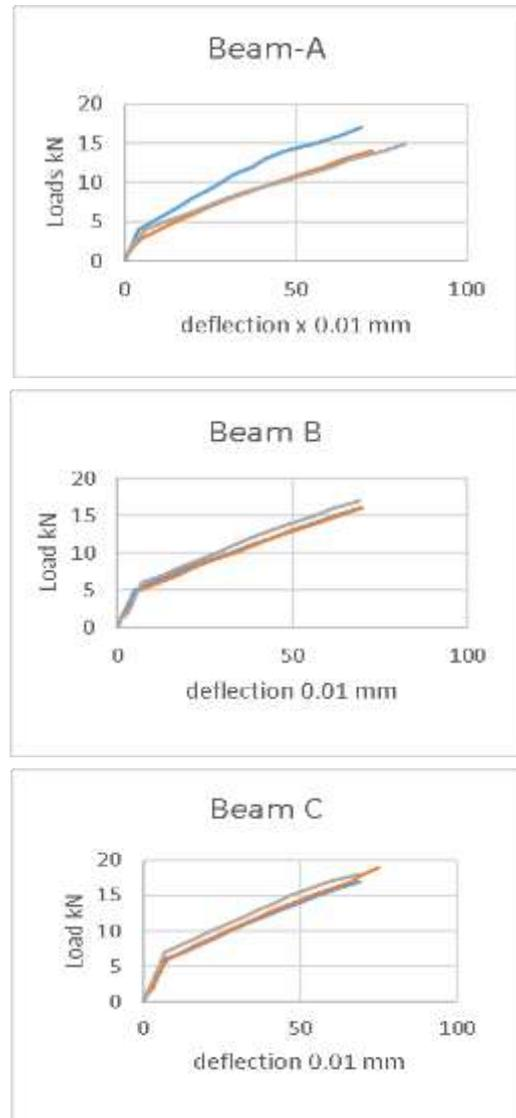
Fig. 4. Load and Deflection Curve
