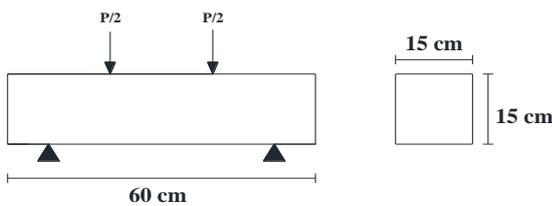
Fig. 2. Beam specimen dimension and loading
