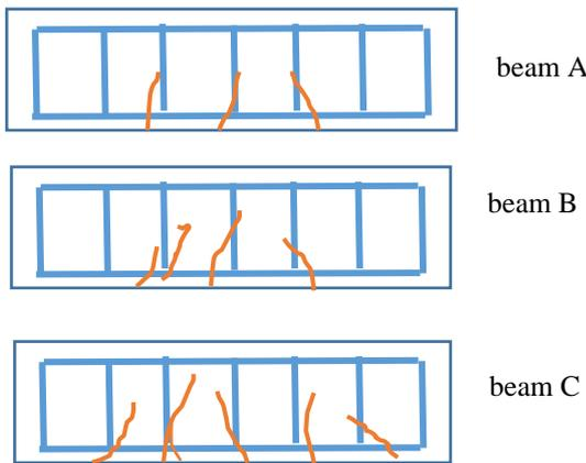
Fig. 5. Crack Pattern of Beam Sample
