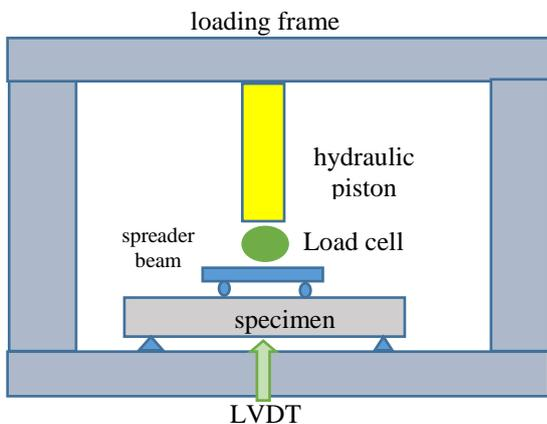
Fig. 3. Loading of beam specimen
