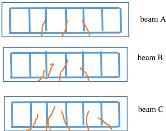
Fig. 5. Crack Pattern of Beam Sample
