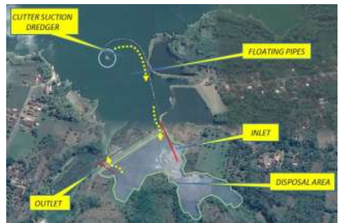
Fig. 4. Scheme of Sutami Reservoir Dredging Work
