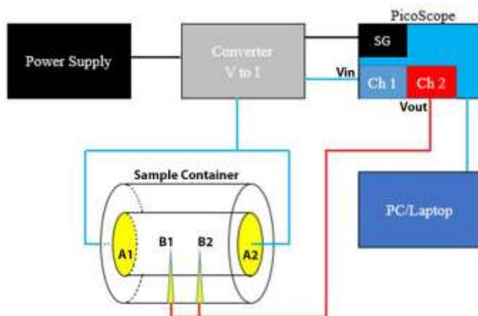
Fig. 1. The electrical impedance measurement system using four electrodes.
