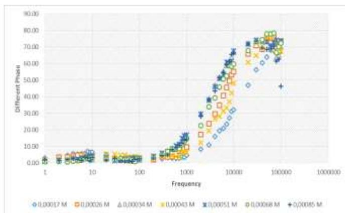
Fig. 3. Differential Phase Graphs to Frequency at seven Variations in NaCl Solution Concentration.
