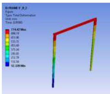
Fig. 10. Total deformation of tapered frame section
