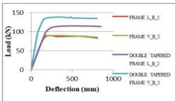
Fig. 11. Comparison of Lateral Load Performance of Tapered Frame Section
