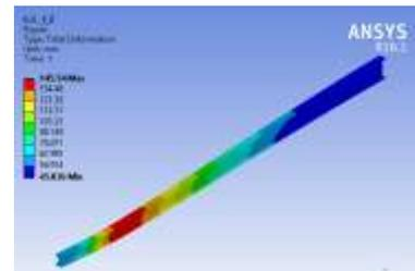
Fig. 4. Total Deformation of Tapered Column
