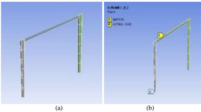
Fig. 9. Geometry and Boundary Conditions of tapered frame section
