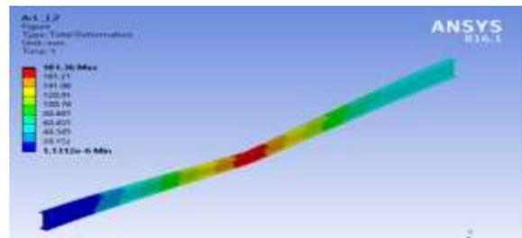
Fig. 7. Total Deformation
