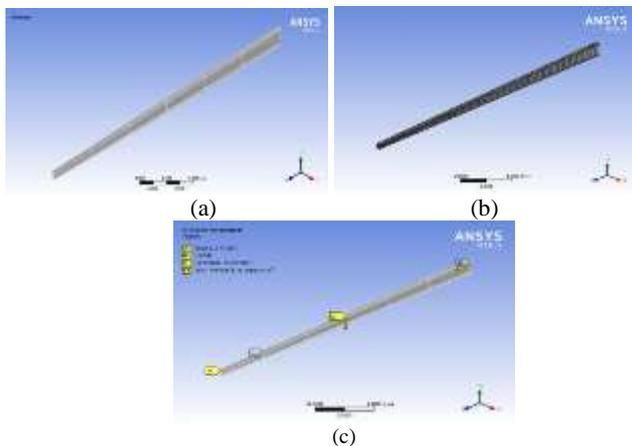
Fig. 3. (a) Isometric view (b) Finite element modeling (c) Boundary conditions of tapered column sections
