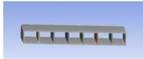
Fig. 2. Cross section of GFRP wall panels-varying thickness & breadth by width ratio (a) varying thickness 3-8mm (b) varying thickness 8-3mm (c) uniform thickness 5mm (d) uniform thickness 4mm and breadth by width ratio 6 (e) uniform thickness 6mm and breadth by width ratio 9
