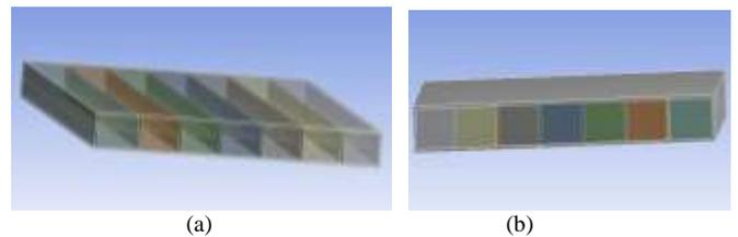
Fig. 5. Cross section GFRP wall panels (a) with rebar (b) without rebar
