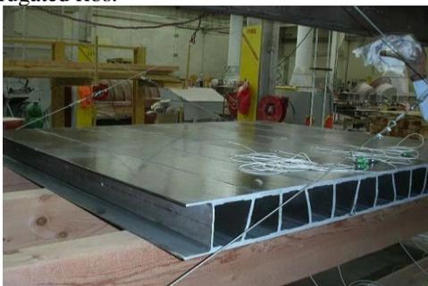
Fig. 1. GFRP deck panel
