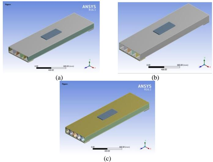
Fig. 3. Cross section of all GFRP deck panels – (a) Rectangular GFRP deck panel with L/D ratio 2 (b) Trapezoidal GFRP deck panel with L/D ratio 2 (c) Elliptical GFRP deck panel with L/D ratio 2
