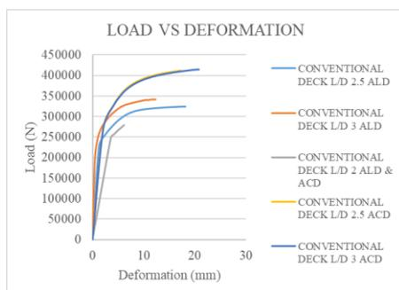
Fig. 9. Load deformation behavior of conventional deck panel along the length and across the width of deck
