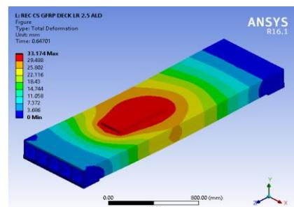
Fig. 4. Total deformation
