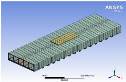
Fig. 7. Finite element modelling of corrugated GFRP deck panels with L/D ratio 2
