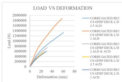
Fig. 8. Load deformation behavior of corrugated GFRP deck panel along the length and across the width of deck
