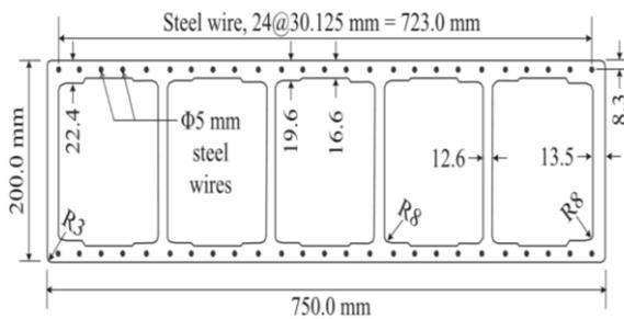
Fig. 2. Cross-sectional profile of steel reinforced GFRP deck panel
