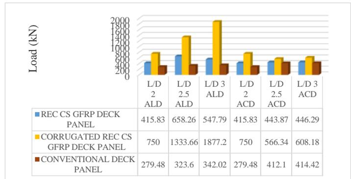
Fig. 10. Ultimate load comparison of deck panel with different L/D ratios
