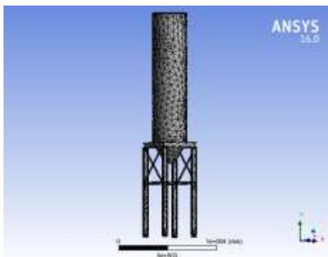
Fig. 2. Meshing on silo with elliptical shaped isolating device
