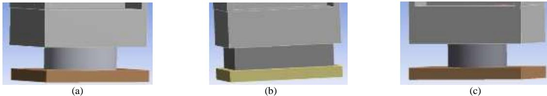
Fig. 1. Cross sections of isolating devices (a) Elliptical shaped isolating device, (b) Rectangular shaped isolating device, (c) Round shaped isolating device
