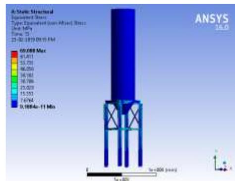
Fig. 3. Equivalent Von-Misses stress of silo with elliptical shaped isolating device
