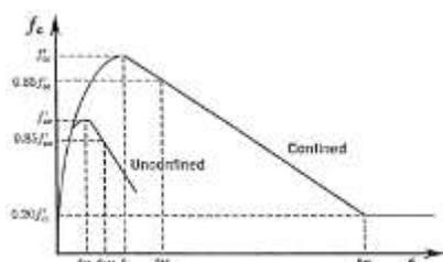
Fig. 2. Proposed stress-strain relationship (Saatcioglu & Razvi, 1999)
