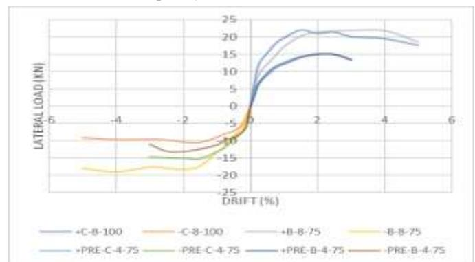
Fig. 2. Envelope curve of specimen lateral load capacity
