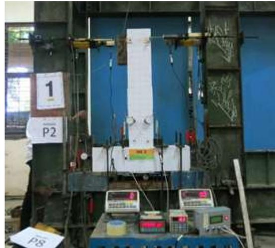
Figure 5. Setting of loading *quasi-cyclic* devices
