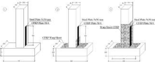
Figure 3. Strengthening grooves of specimens
