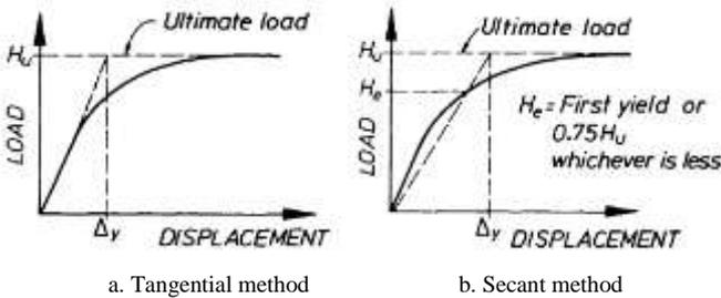
Figure 7. Method for determining the yield point when Pmax
