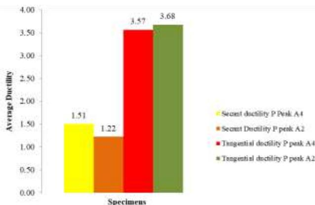
Fig. 5. The results of the comparison of tangential ductility and secant ductility in P peak on 4 specimens
