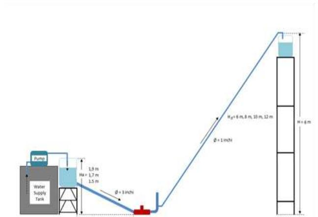
Fig. 3. Installation hydraulic ram pump
