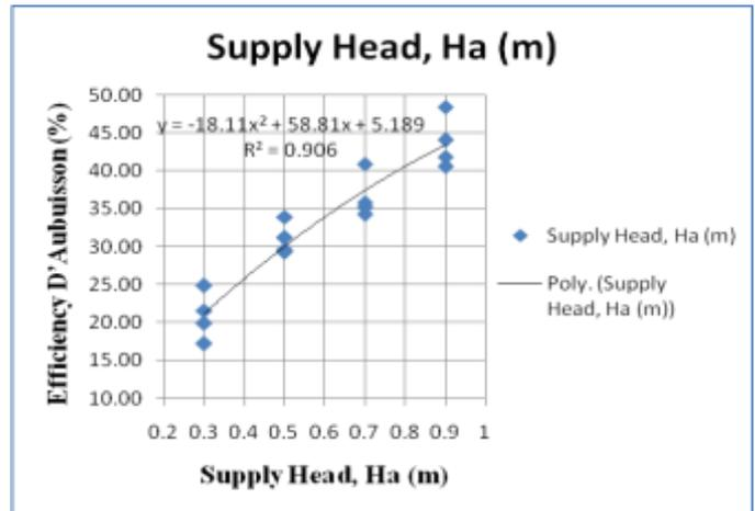
Fig. 6. Relationship between supply head, Ha (m) and efficiency D'Aubuisson for each delivery pipe length
