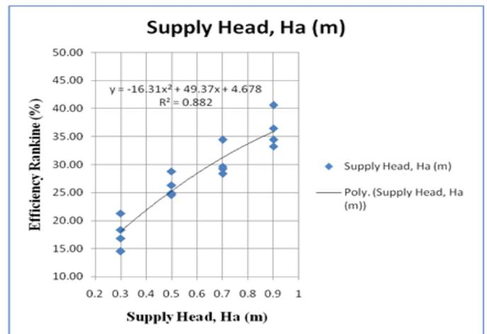
Fig. 7. Relationship between supply head, Ha (m) and efficiency Rankine for each delivery pipe length
