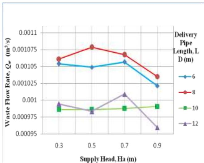
Fig. 4. Relationship between supply head and waste flow rate for each delivery pipe length variation
