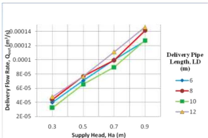
Fig. 5. Relationship between supply head and delivery flow rate for each delivery pipe length variation.
