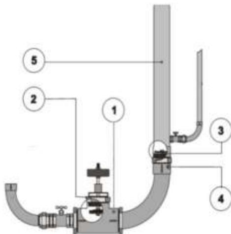
Fig. 2. The main component of the ram hydraulic pump, 1) Valve box (2) Waste valve (3) Delivery valve (4) Air valve, (5) Air vessel
