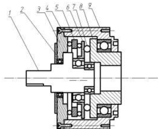
Fig. 1. Transmission principle of the cycloid steel ball reducer
