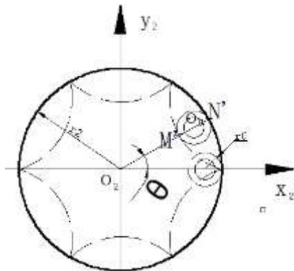
Fig. 3. Generation principle of hypocycloid
