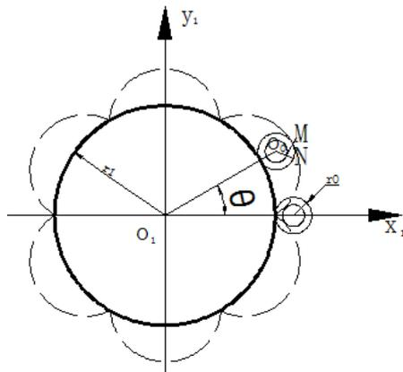
Fig. 2. Generation principle of epicycloid
