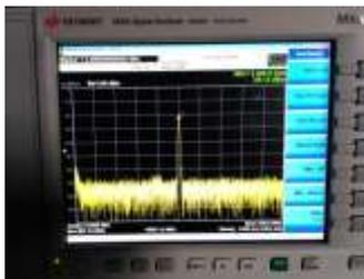
Fig. 19. Signal receive on micro-strip antenna shown in signal analyzer
