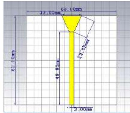
Fig. 2. Shape and Dimension of Antenna
