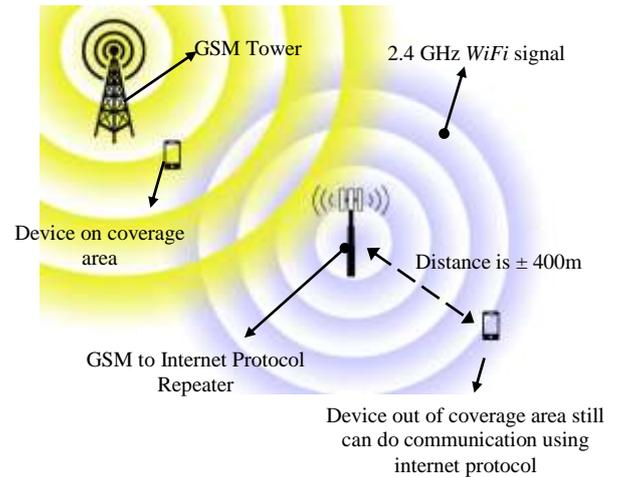
Fig. 20. Schematic of blank-spot area
