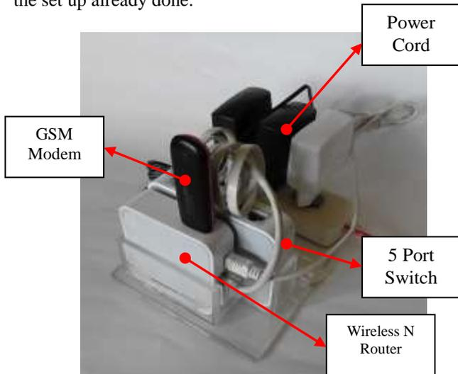
Fig. 22. GSM to internet protocol converter
