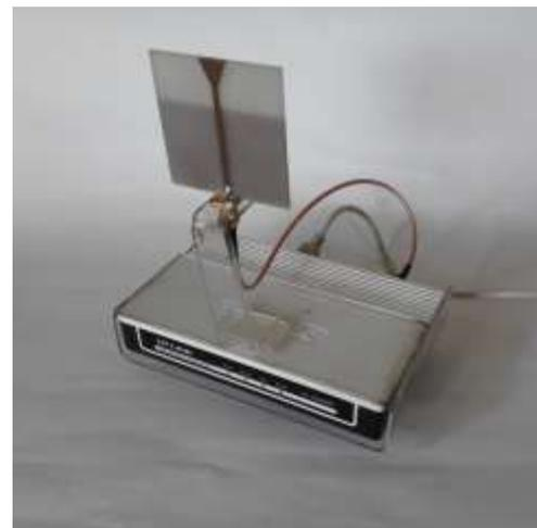
Fig. 21. Antenna connected to Wi-Fi Router
