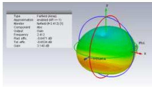
Fig. 9. Radiation pattern on 3D
