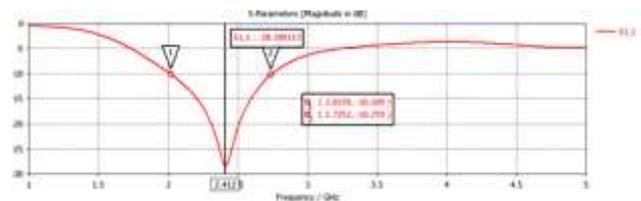
Fig. 4. S Parameter Antenna Simulation
