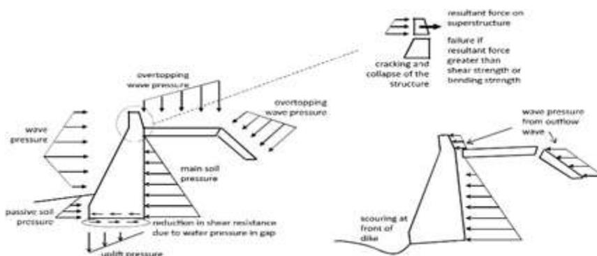
Figure 4: Caisson breakwater section (a) former design (b) recommended design for a 'strong breakwater' able to resist a tsunami beyond the design height (based upon [44]).
