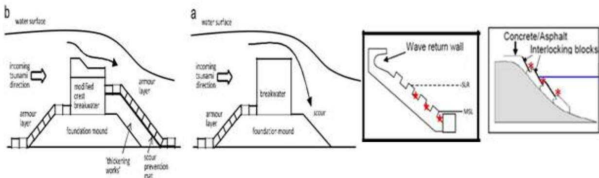
Figure 3: Modified drawing of a seawall with a structure that helps the return of the waves
