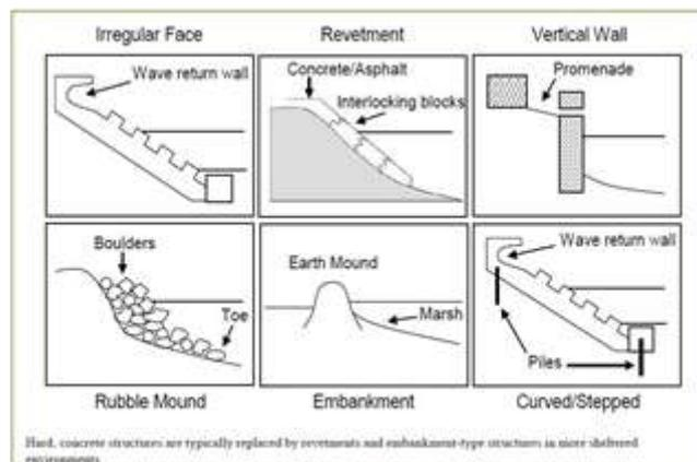
Figure 2: Variation in design types of seawalls. Source: Adapted by Linham and Nicholls (2010) from French, (2001)
