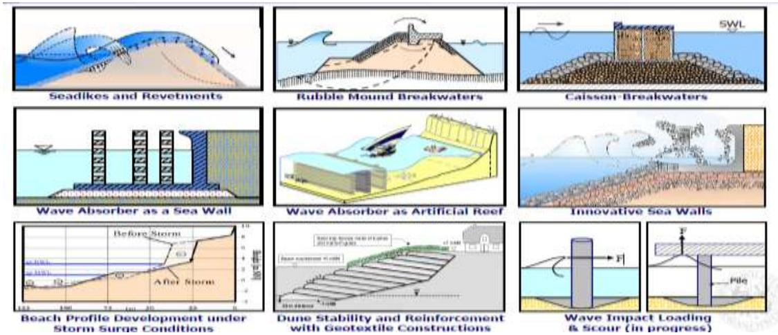
Furthermore, as indicated in the Figure 2, if seawalls could be coupled with soft barriers and such soft barriers could be artificially transplanted within the irregular depressions on the hard defense structures or if they could be designed to give a terraced appearance, such structures will enhance the effect of hard structures against wave action.
