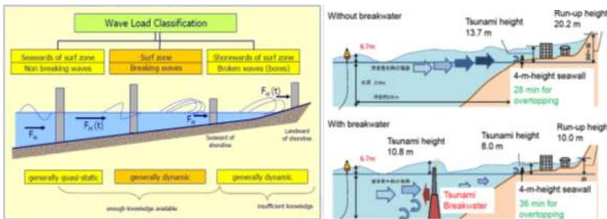
Figure 9: Tsunami impact reduction performance of the Kamaishi breakwaters (PARI, 2011)
