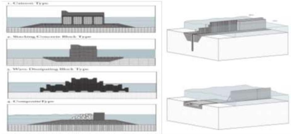
Figure 8: Breakwaters with vertical and inclined concrete walls
