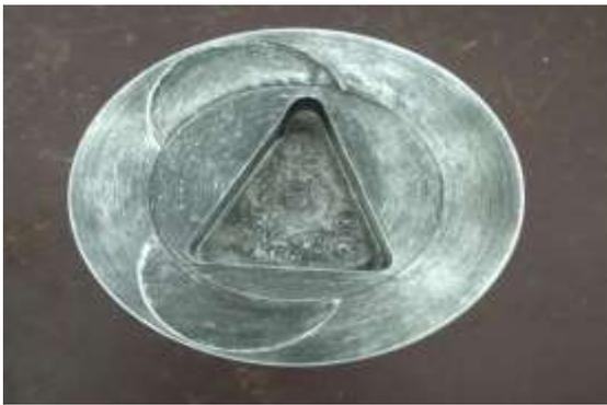
Fig. 2. Triangular Piston Crown
