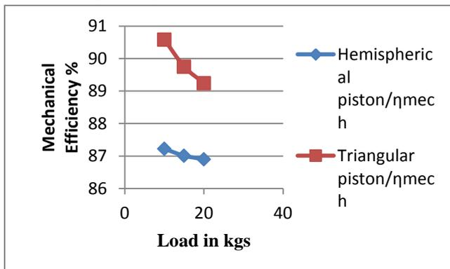
Fig. 7. Comparison of Mechanical efficiency
