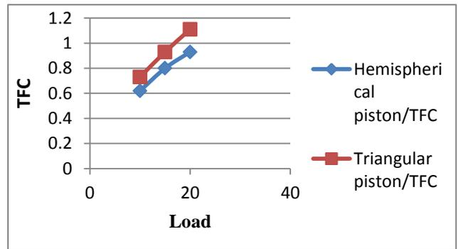
Fig. 3. Comparison of TFC Vs Load
