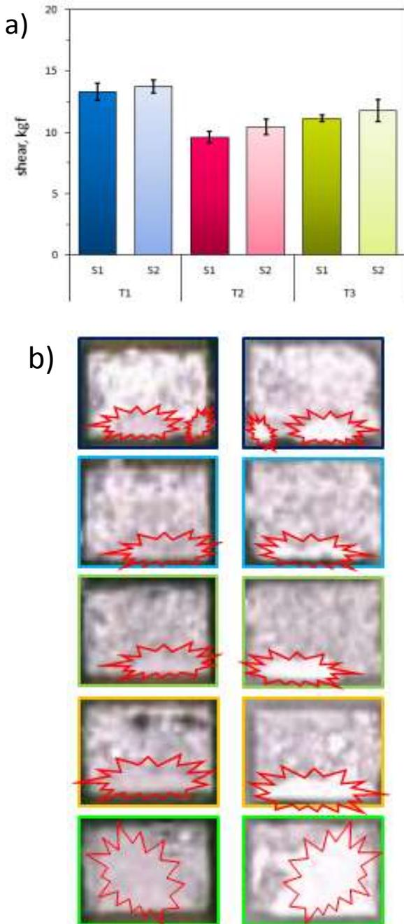
Fig. 1. a) Shear strength of soldered system subjected to three thermal treatments. b) Sheared surfaces showing significant interfacial fractures (enclosed).
