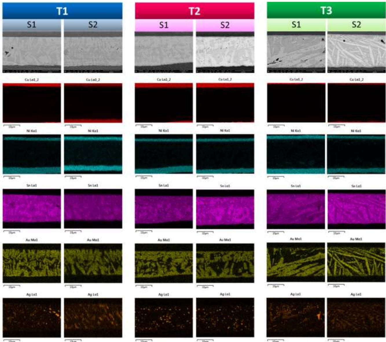
Fig. 2. SEM images and EDS maps of the sandwiched solder cross-sectioned surfaces. Cu - red, Ni - blue green, Sn - violet, Au - yellow, and Ag - orange.
