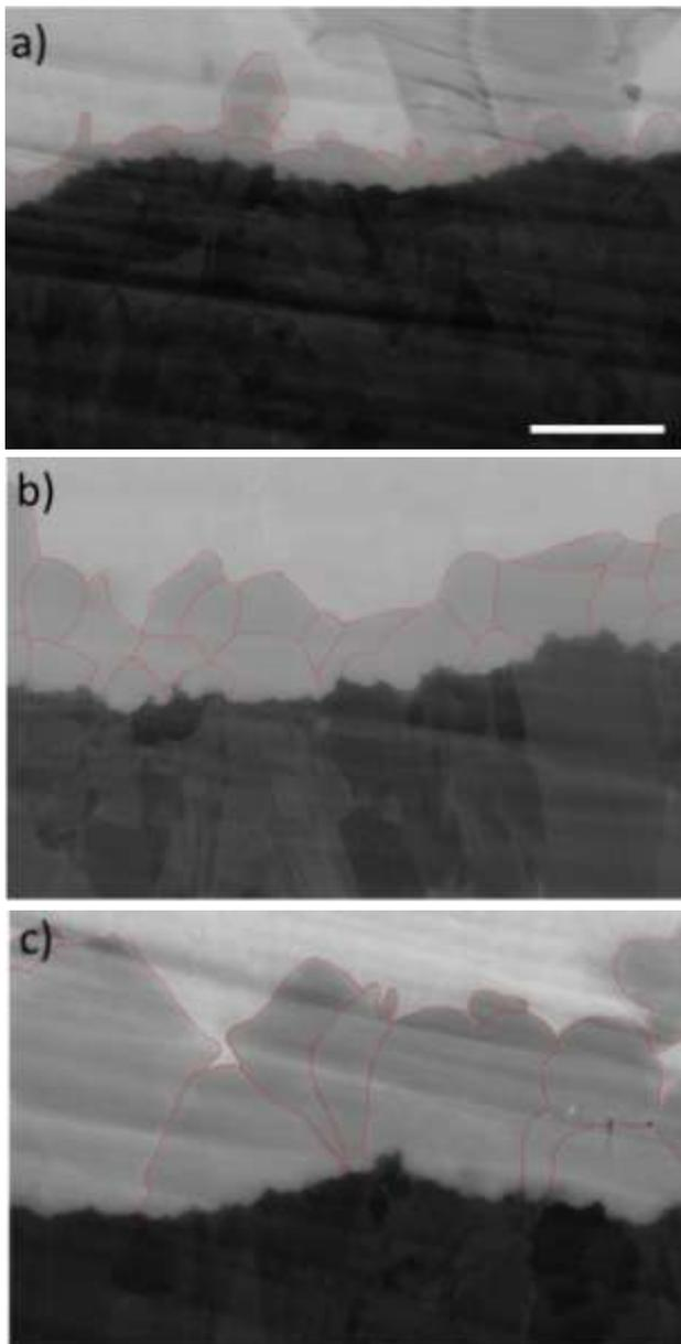
Fig. 4. IMC growth after the thermal treatments; a) T1, b) T2, and c) T3.
