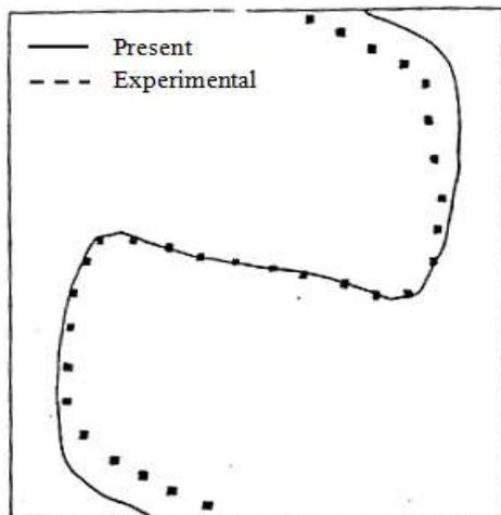
Fig. 9. Dimensionless of the isothermal contour lines of 0.5 with the published results, [5] for the enclosure containing a square cavity,  $Ra^* = 0.64 \times 10^6$ ,  $Pr = 0.71$ ,  $K^* = 7.4$ ,  $A^* = 0.36$ ,  $AS = 1.0$ ,  $AS1 = 1.0$ ,  $\theta = 90^\circ$ .
