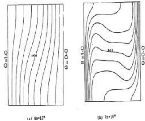
Fig. 4. Dimensionless isothermal contour lines for enclosure with perfectly insulated connecting walls, Pr=0.71, AS1=1.0,  $\Delta\theta = 0.1$ .
