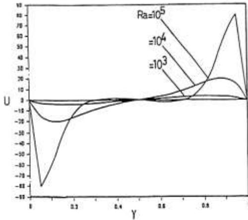
Fig. 6-a. Dimensionless vertical velocity components at horizontal mid-plane, for enclosure with perfectly insulated connecting walls,  $Pr=0.71$ ,  $AS1=1.0$ , and  $\phi=90^\circ$ .
