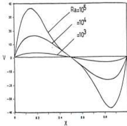
Fig. 6-b. Dimensionless horizontal velocity components at horizontal mid-plane, for enclosure with perfectly insulated connecting walls,  $Pr=0.71$ ,  $AS1=1.0$ , and  $\phi=90^\circ$ .
