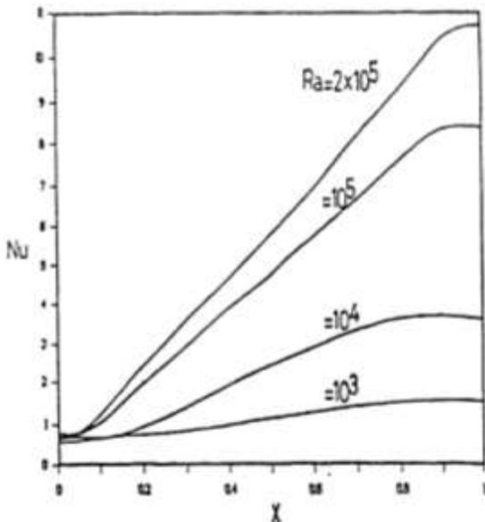
Fig. 7. Distribution of the local Nusselt numbers at the heated wall for enclosure with perfectly insulated connecting walls,  $Pr=0.71$ ,  $AS1=1.0$ , and  $\phi=90^\circ$ .
