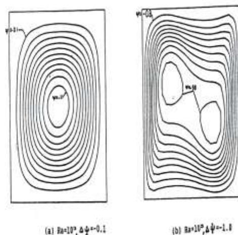
Fig. 5. Dimensionless streamlines for enclosure with perfectly insulated connecting walls, Pr=0.71, AS1=1.0,  $\Delta\psi = 1=90^\circ$ .
