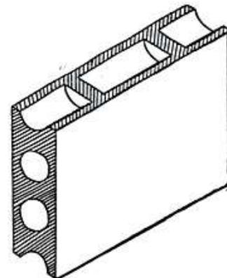
Fig. 2. Truncated circular cylinder cavities.
