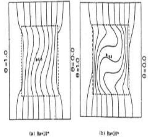
Fig. 8. Dimensionless isothermal contour lines for enclosure containing a square cavity,  $Pr=0.71$ ,  $K^*=10.0$ ,  $A^*=0.36$ ,  $AS=1.0$ ,  $AS1=1.0$ ,  $E=0$ ,  $\phi=90^\circ$  and  $\Delta\theta=0.1$ .
