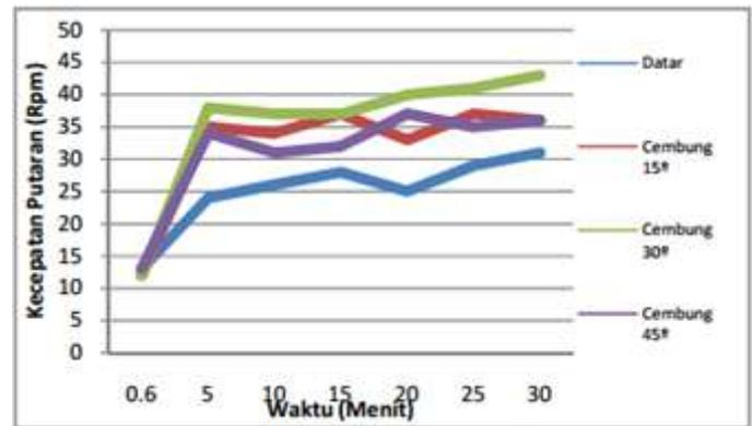
Fig. 5. Graph the turbine rotation ratio at wind speed 6 m / s loaded.
