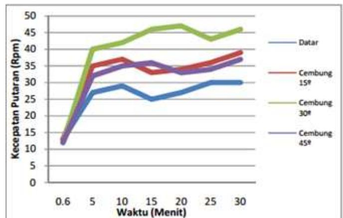
Fig. 6. Graph the turbine rotation ratio at wind speed 7 m / s loaded.
