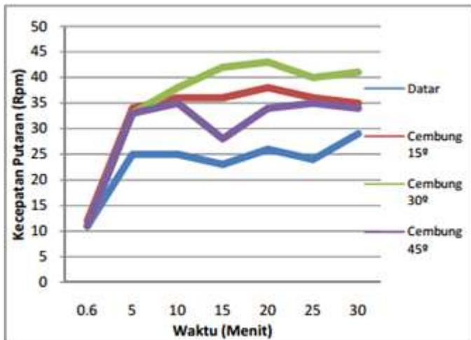
Fig. 4. Graph the turbine rotation ratio at wind speed 5 m / s loaded.
