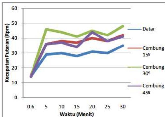
Fig. 7. Graph the turbine rotation ratio at wind speed 10 m / s loaded.
