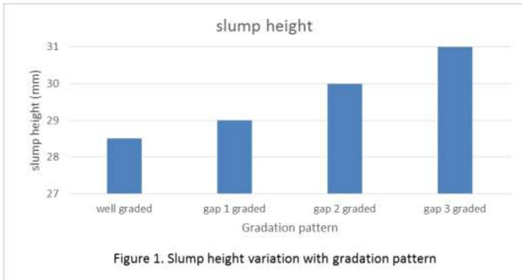
Figure 1. Slump height variation with gradation pattern
