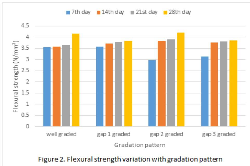
Figure 2. Flexural strength variation with gradation pattern
