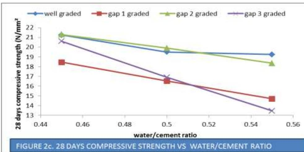
For 28<sup>th</sup> day, 0.45 w/c ratio concrete, the mean compressive strength were 21.25N/mm<sup>2</sup>, 18.45N/mm<sup>2</sup>, 21.30
