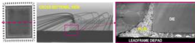
Fig. 1. Cross-sectional view of the leadframe package.
