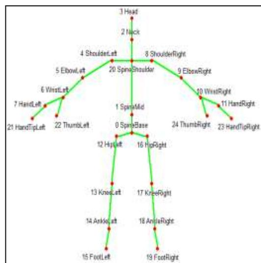
Fig. 3. 25 tracked Joints by Kinect SDK.
