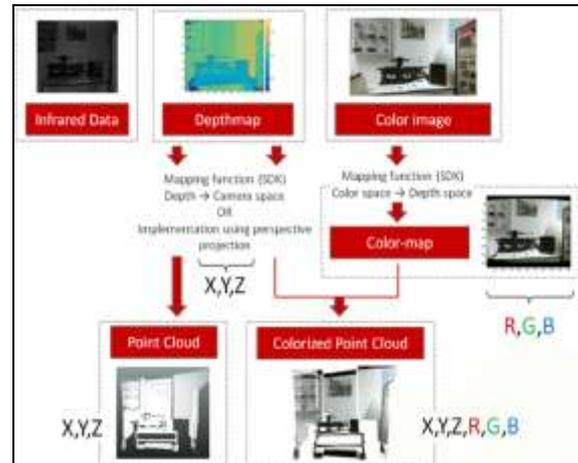
Fig. 2. Data Streams Generated by Kinect V2.
