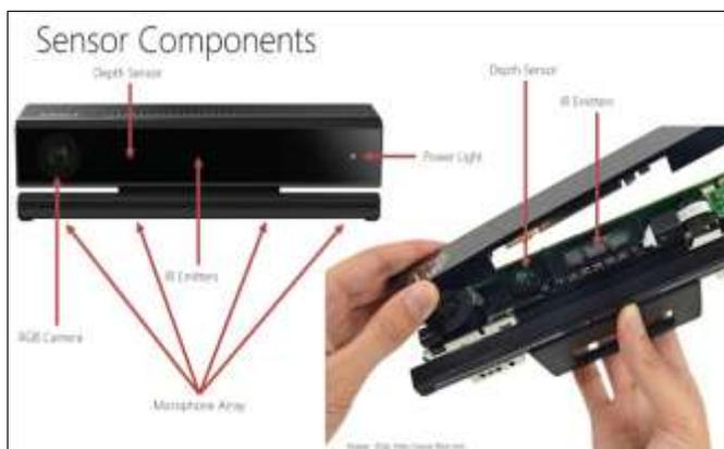
Fig. 1. Sensors in Microsoft Kinect v2.
