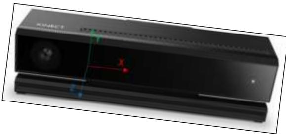
Fig. 4. 3D Coordinate placement on the Kinect Sensor.
