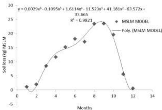
Figure 6: Calibration of MSLM of 6 Order Polynomial
