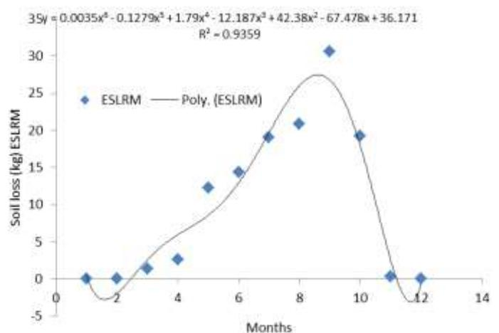
Figure 5: Calibration of ESLRM of 6 Order Polynomial
