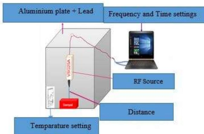
Fig. 3. RF exposure process in the sample.
