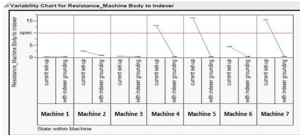
Fig. 11. Resistance reading, before and after implementing machine grounding.
