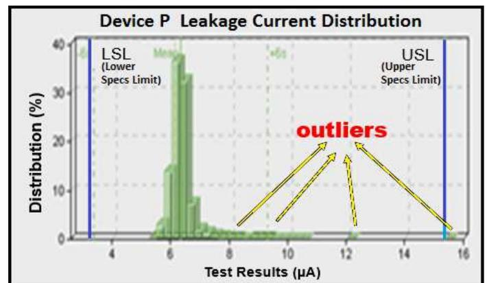
Fig. 1. Leakage current PPAT response, showing the outliers.
