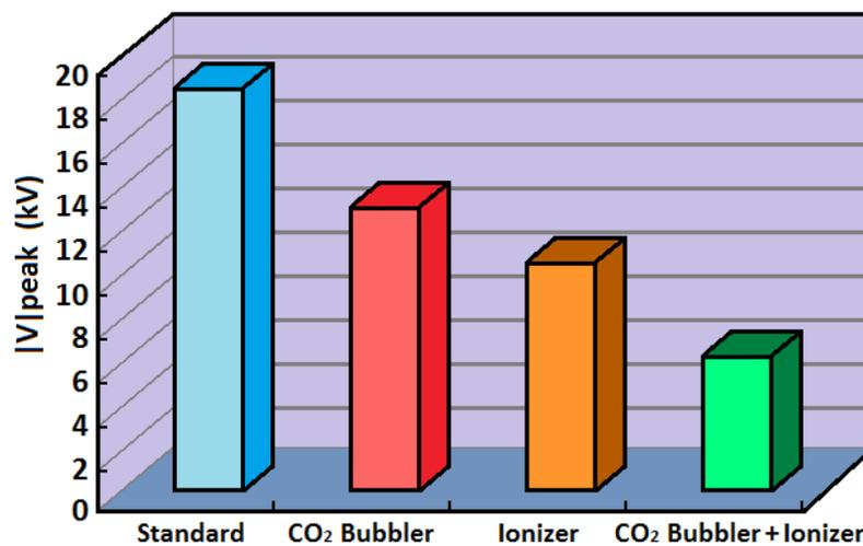
Fig. 7. Discharge voltage at wafer saw process [6].
