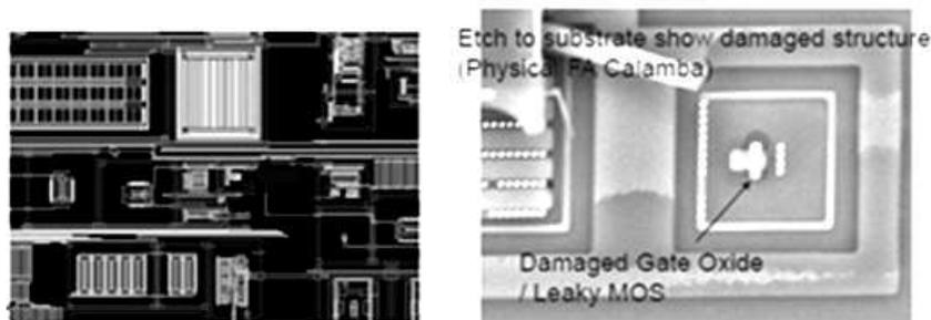
Fig. 6. Damage gate oxide with plasma process [3].
