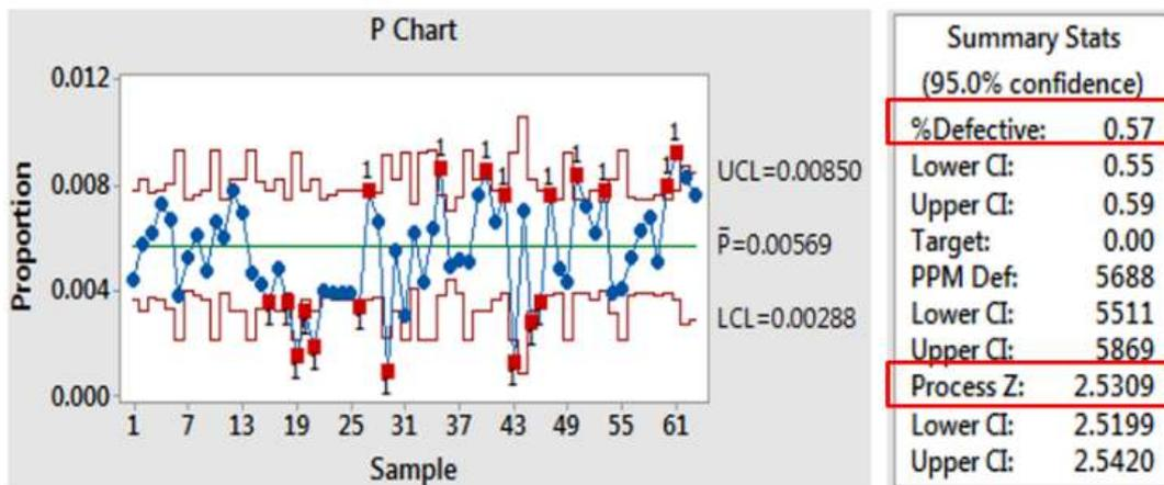
Fig. 4. Current process capability.
