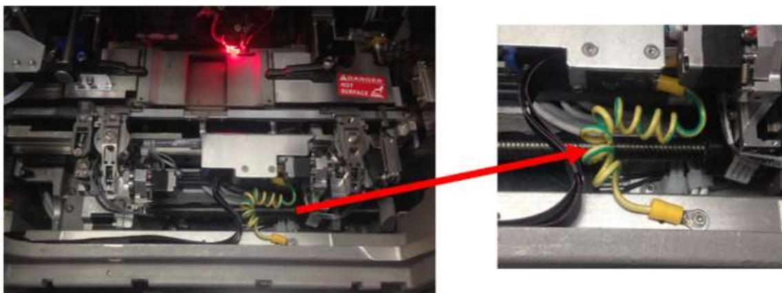
Fig. 10. Wirebond workholder machine grounding.
