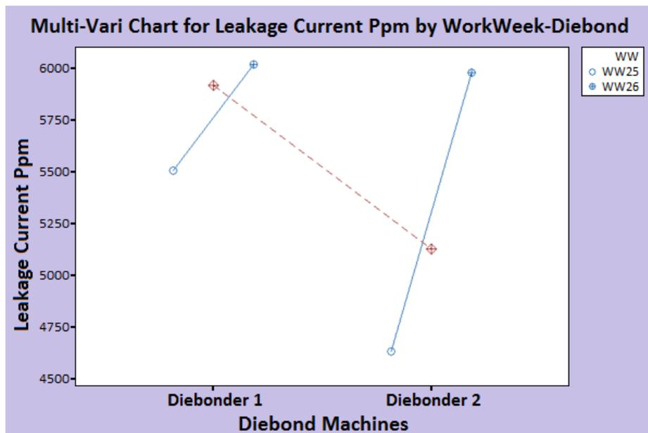
Fig. 9. Multi-vari analysis on diebond machines.
