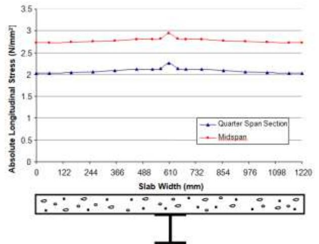
Fig. 6. Slab top surface stress distribution for Yam and Chapman beam for LL (18.228 kN/m).
