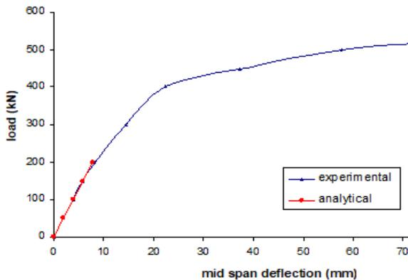
Fig. 4. Yam and Chapman composite steel concrete beam experimental and analytical load-deflection curve.
