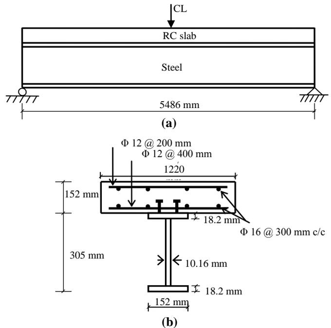
Fig. 2. Yam and Chapman tested beam (a) dimensions and loading arrangement of beam (b) cross section [18].
