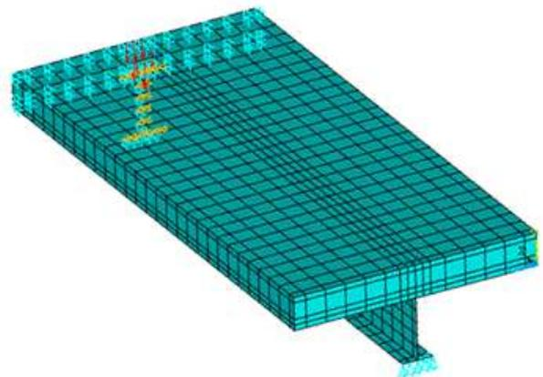
Fig. 3. Finite element idealization for Yam and Chapman composite steel concrete beam.
