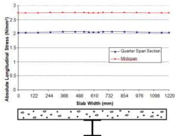
Fig. 7. Slab top surface stress distribution for Yam and Chapman beam for UDL (14.941 kN/m<sup>2</sup>).
