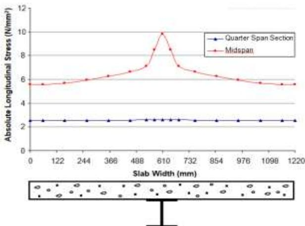
Fig. 5. Slab top surface stress distribution for Yam and Chapman beam for CL (100 kN).
