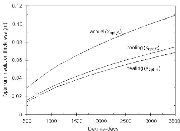
Fig. 5. Variation of optimum insulation thicknesses with degree-days.
