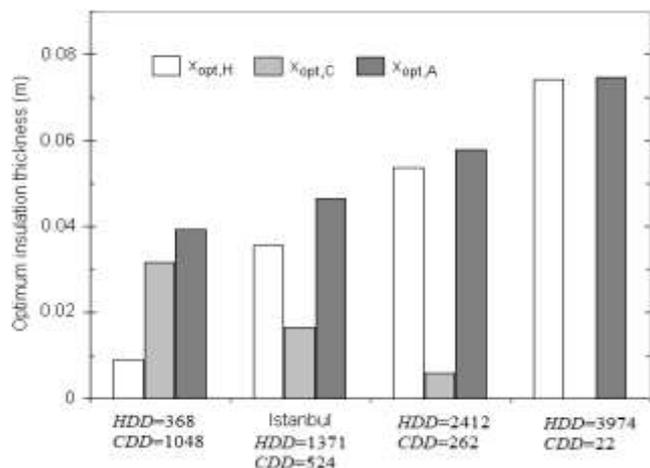
Fig. 4. The optimum insulation thicknesses considering heating, cooling and annual energy requirements.
