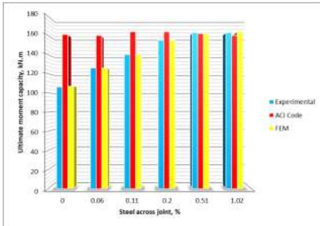
Fig. 5. Variation of ultimate moment capacity with steel percentage across the joint.
