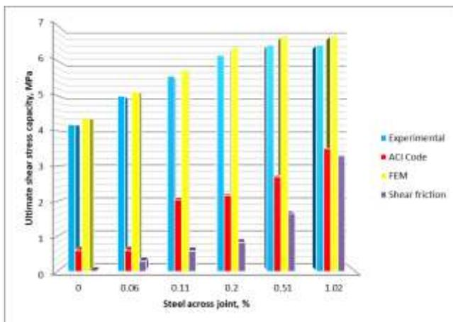
Fig. 6. Variation of ultimate shear stress with steel percentage across the joint.
