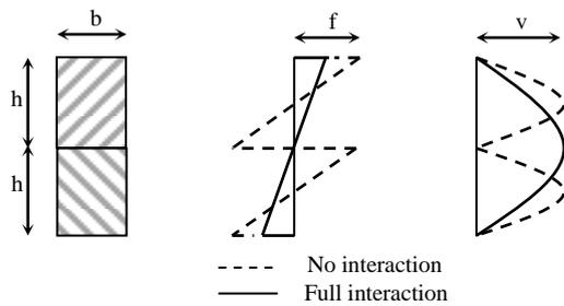
a. section b. bending stress c. shearing stress
