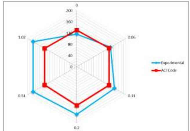
Fig. 7. Comparison between the experimental and ACI ultimate shear strength with steel percentage across the joint.
