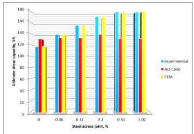
Fig. 4. Variation of ultimate shear capacity with steel percentage across the joint.
