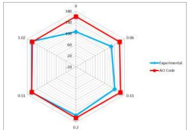
Fig. 8. Comparison between the experimental and ACI ultimate bending moment strength with steel percentage across the joint.
