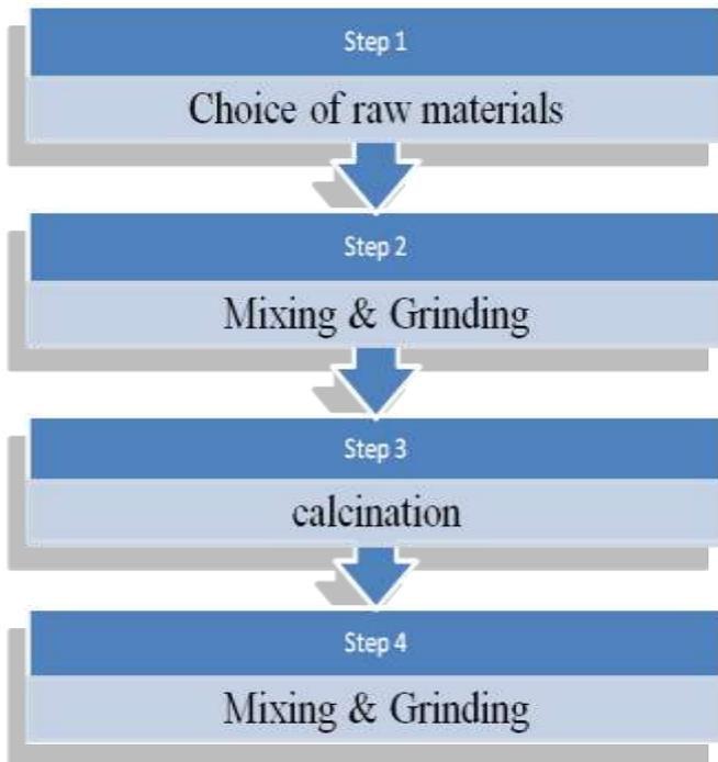
Fig. 2. Main steps in the manufacture of  $Sr_{2(1-x)}Na_{(1+x)}Gd_xNb_5O_{15}$
