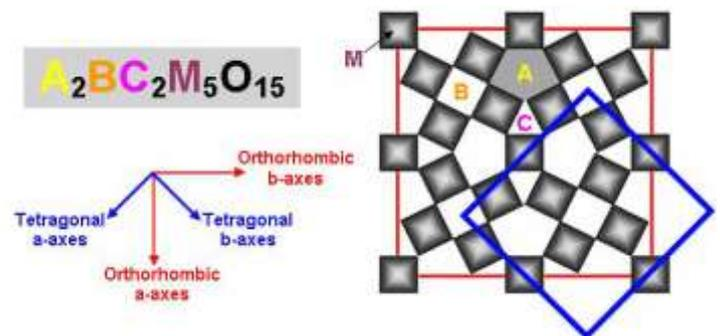
Fig. 1. Schematic projection of the TTB crystalline network along the fourfold c axis (A, B and C correspond to cationic sites with coordination number 15, 12 and 9, respectively, in the unit cell  $\text{A}_2\text{BC}_2\text{M}_5\text{X}_{15}$ ).
