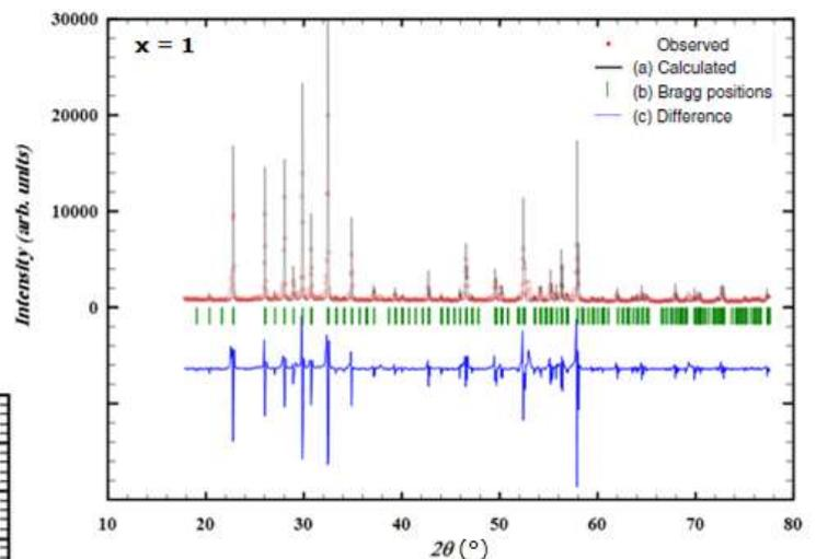
Fig. 3. Observed, calculated and difference X-ray diffraction patterns for compounds with  $x=0$ ,  $x=0.8$  and  $x=1$ .
