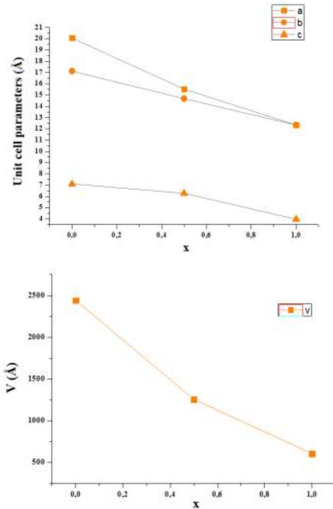
Fig. 4. Evolution of the lattice parameters and volume of  $Sr_{2(1-x)}Na_{(1+x)}Gd_xNb_5O_{15}$  as a function of the gadolinium content  $x$ .
