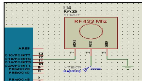
Fig. 4. Transmitter circuit.
