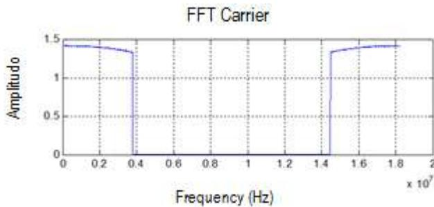
Fig. 7. Frequency response of signal carriers 8K mode.
