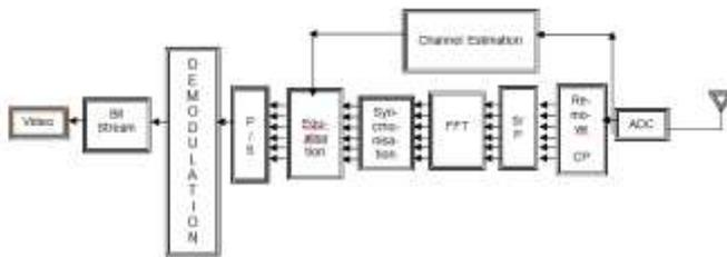
Fig. 15. Receiver design system DVB-T2 using OFDM.
