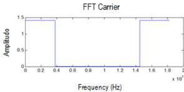
Fig. 6. Frequency response of signal carriers 2K mode.
