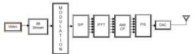
Fig. 3. Transmitter design system DVB-T2 using OFDM.
