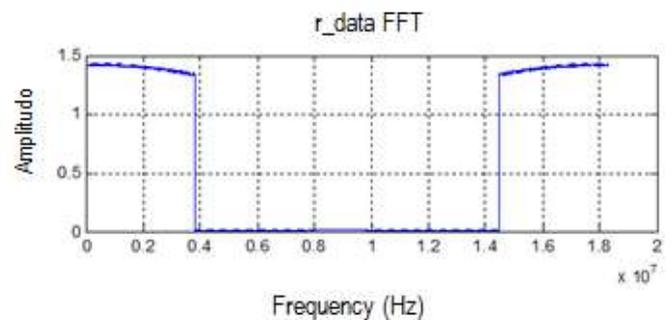
Fig. 19. Frequency response of signal output 8K mode.
