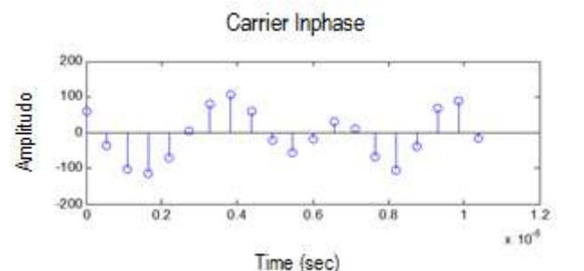
Fig. 5. Time response of signal carriers 8K mode.
