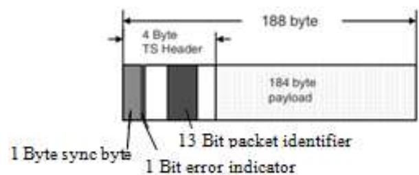
Fig. 1. MPEG2 Transport stream packets.
