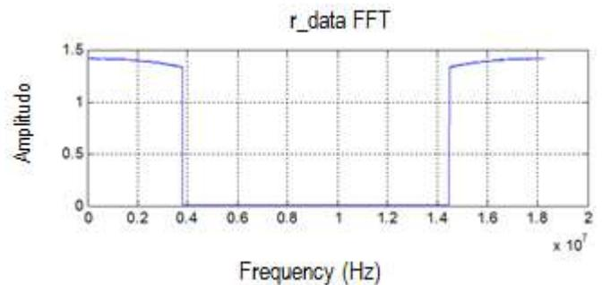
Fig. 18. Frequency response of signal output 2K mode.
