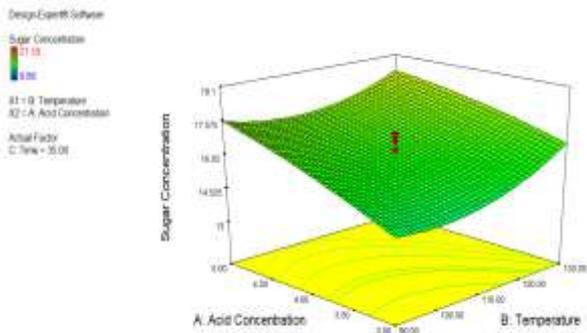
Fig. 3.4b. Response surface plot showing the effect of acid concentration and temperature on the total reducing sugar concentration.
