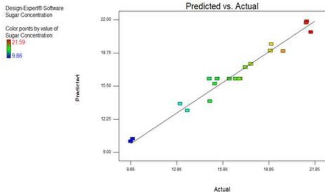
Fig. 3.3. Predicted vs Actual response values for the quadratic model fit for the dilute acid hydrolysis of sugarcane bagasse.
