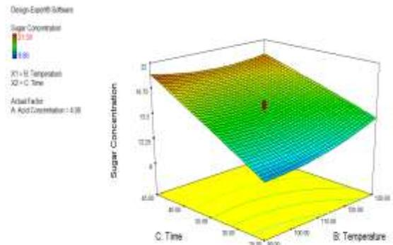
Fig. 3.6b. Response surface plot showing the effect of reaction time and hydrolysis temp. on the total reducing sugar concentration.
