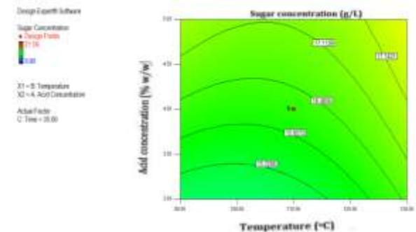
Fig. 3.4a. Contour plot showing the effect of acid concentration and temperature on the total reducing sugar concentration.
