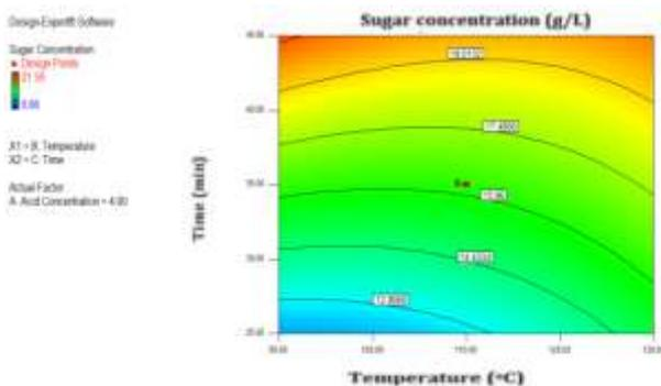
Fig. 3.6a. Contour plot showing the effect of reaction time and hydrolysis temperature on the total reducing sugar concentration.
