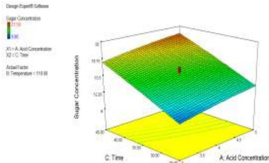
Fig. 3.5b. Response surface plot showing the effect of reaction time and acid concentration on the total reducing sugar concentration.
