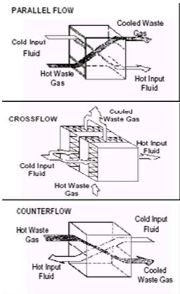
Fig. 4. Sketch for three types of heat exchanger.
