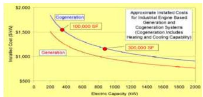
Fig. 8. Effect of engine-based CHP system capacity on installed.
