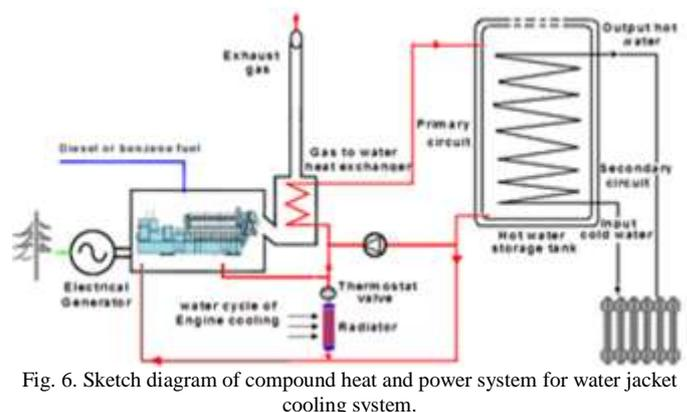
Fig. 6. Sketch diagram of compound heat and power system for water jacket cooling system.
