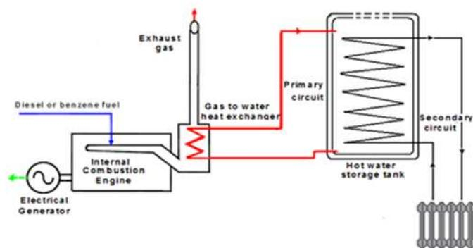
Fig. 7. Sketch diagram of combined heat and power for air cooling engine.
