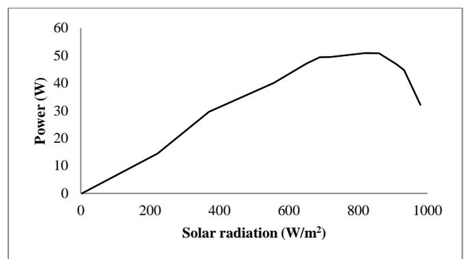
Fig. 6. Solar radiation impact on the generated power.
