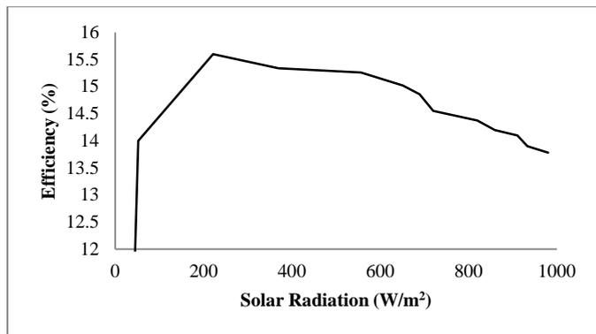
Fig. 7. PV efficiency variation with solar radiation.
