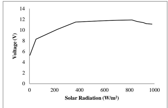
Fig. 5. The impact of solar radiation on voltage.
