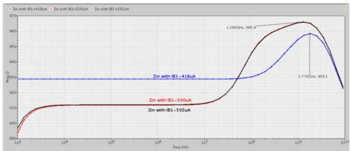
Fig. 7. Simulated impedance-frequency characteristics of the fig. 3 for three different values of I_{B1} .
