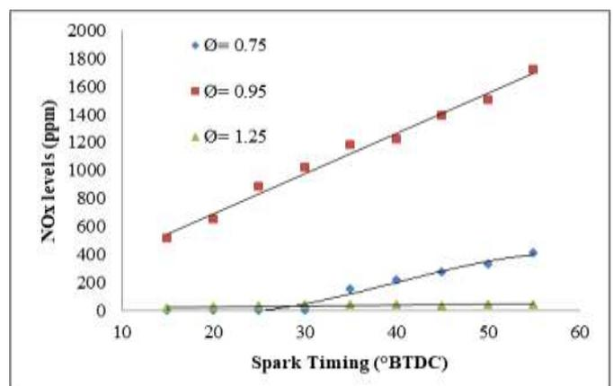
Fig. 3. The impact of spark timing variation on the NOx levels for three specific equivalence ratios.
