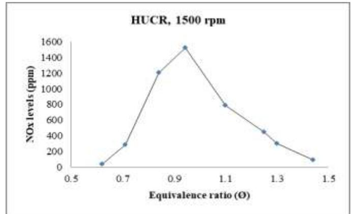
Fig. 2. The impact of equivalence ratio variation on emitted NOx levels.
