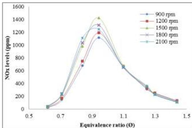
Fig. 5. The impact of engine speed variation on the NOx levels for wide range of equivalence ratio.
