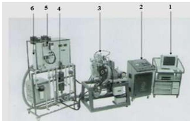
1. Computer and its accessories 2. Control panel 3. The engine 4. Engine's cooling unit 5. The engine's fuel unit 6. The air supply system
