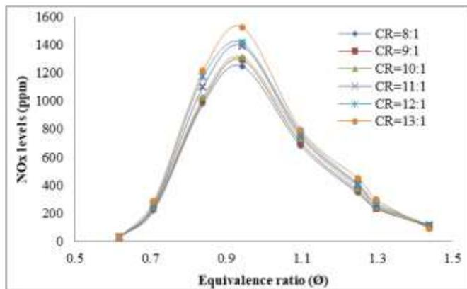
Fig. 4. The impact of compression ratio variation on NOx levels for wide range of equivalence ratios.
