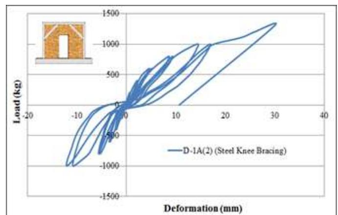
Fig. 5. Load-deformation relationship of cyclic load test of wall with steel knee bracing.
