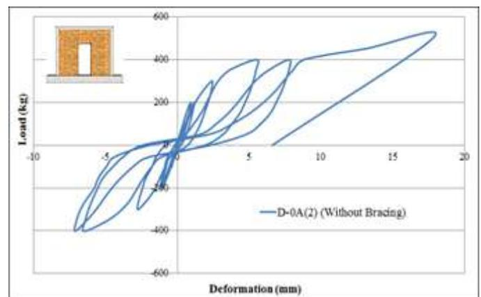
Fig. 4. Load-deformation relationship of cyclic load test of wall without bracing.
