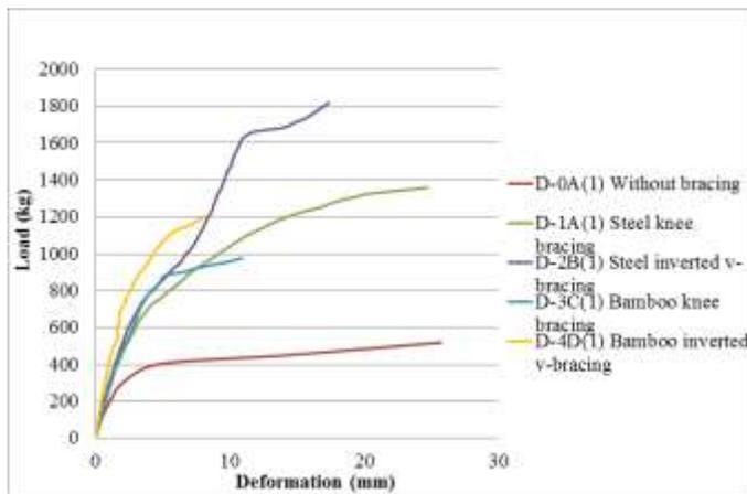
Fig. 3. Load-deformation relationship of wall monotonic test.
