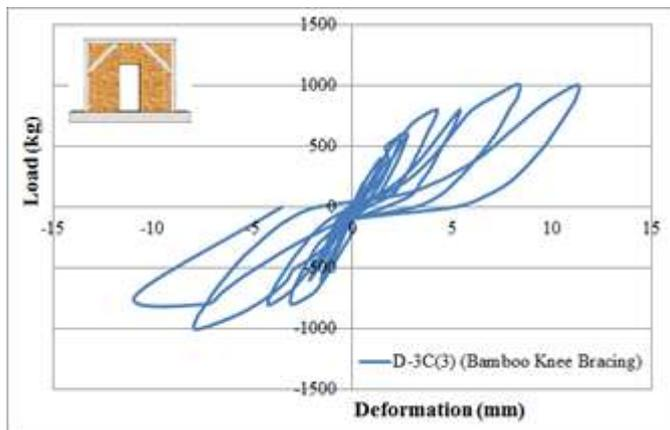
Fig. 7. Load-deformation relationship of cyclic load test of wall with bamboo knee bracing.
