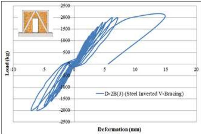
Fig. 6. Load-deformation relationship of cyclic load test of wall with steel inverted v-bracing.
