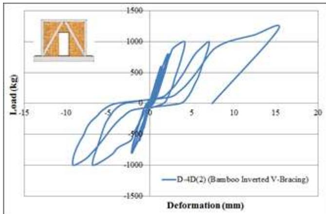
Fig. 8. Load-deformation relationship of cyclic load test of wall with bamboo inverted v-bracing.
