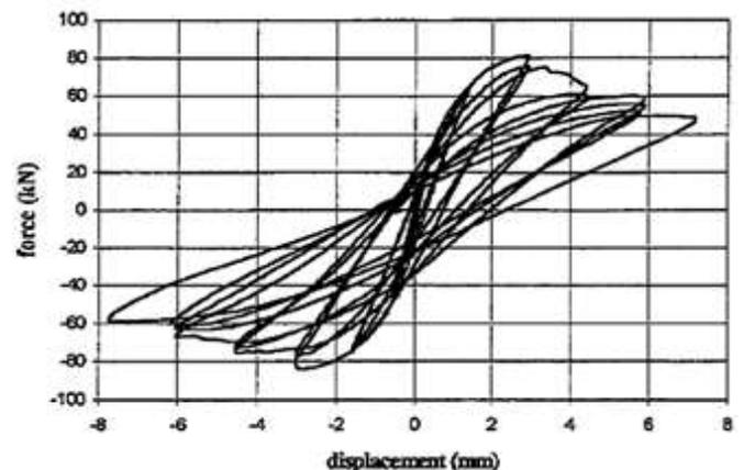
Fig. 1. Hysteretic curve behavior because of diagonal shear crack [4].
