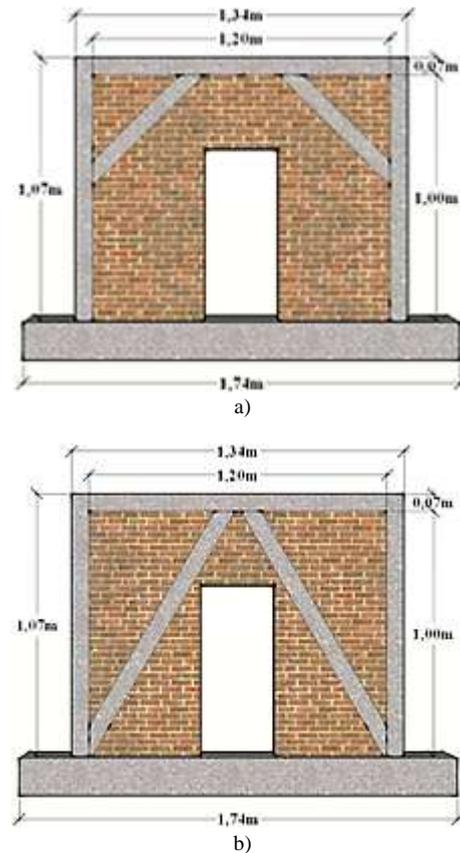
Fig. 2. Specimen model a) Knee bracing b) Inverted v-bracing.
