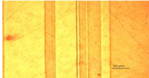
Fig. 5. Lamellar growth along axis of ingot.
