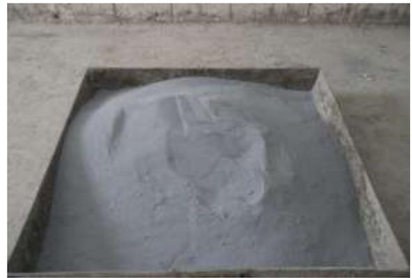
Fig. 2. Silica fume sample.
