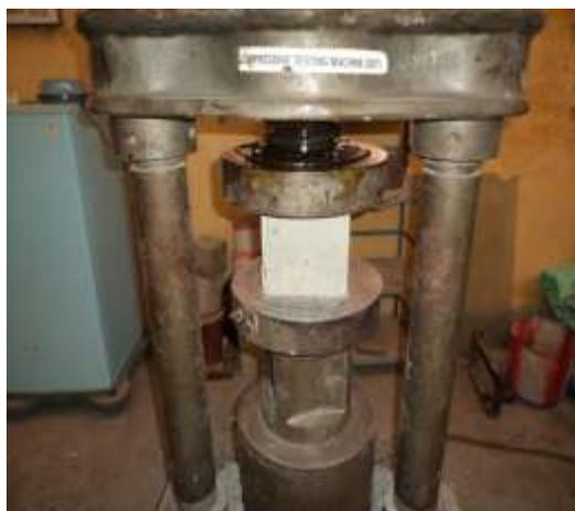
Fig. 4. Cube compression test.
