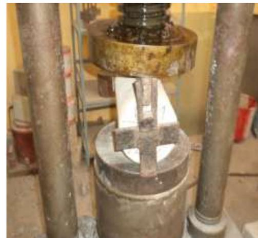
Fig. 5. Split tensile strength.
