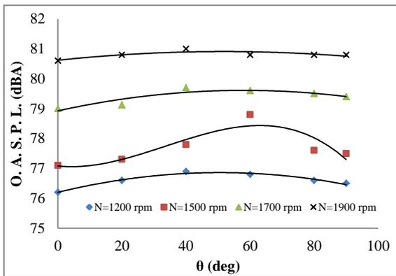
Fig. 6. The impact of engine's velocity variation on the emitted noise for 20% methanol added to gasoline.
