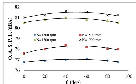
Fig. 5. The impact of engine's velocity variation on the emitted noise for 10% methanol added to gasoline.
