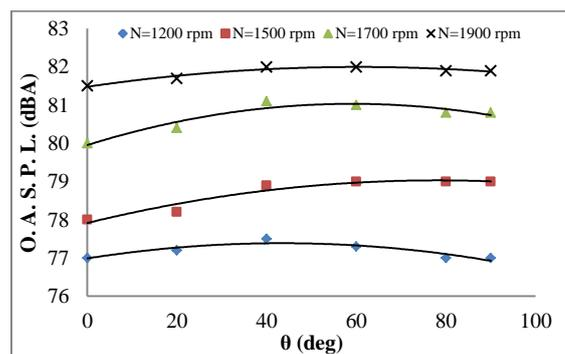
Fig. 4. The impact of engine's velocity variation on the emitted noise for gasoline.
