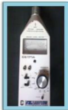
Fig. 2. Illustration of noise measurement device.
