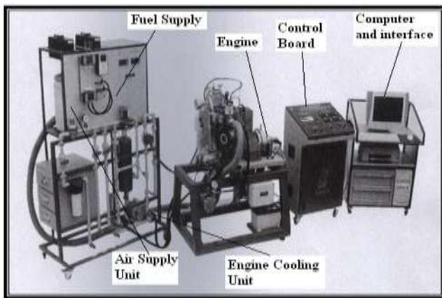
Fig. 1. Illustration of the engine kit and its accessories used in the study.
