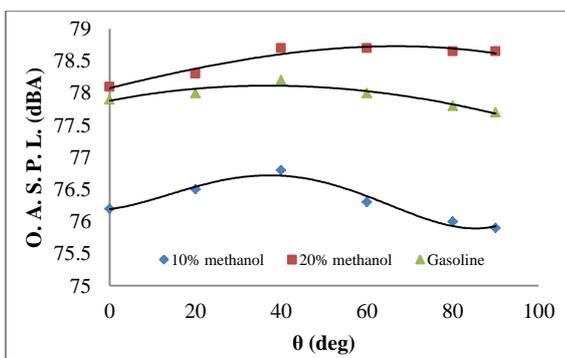
Fig. 3. The impact of adding methanol to gasoline on emitted noise at 1500 rpm.
