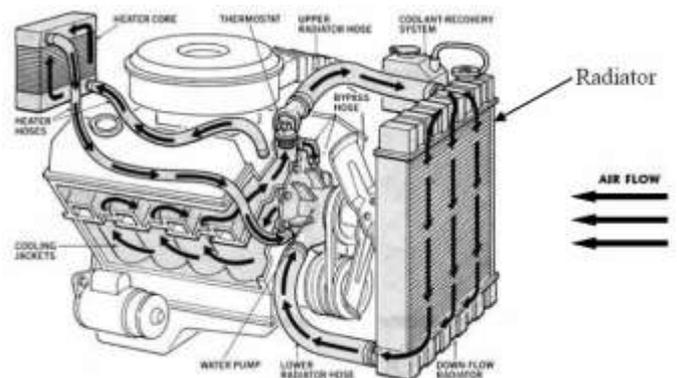
Fig. 1. Schematic of radiator [4]
