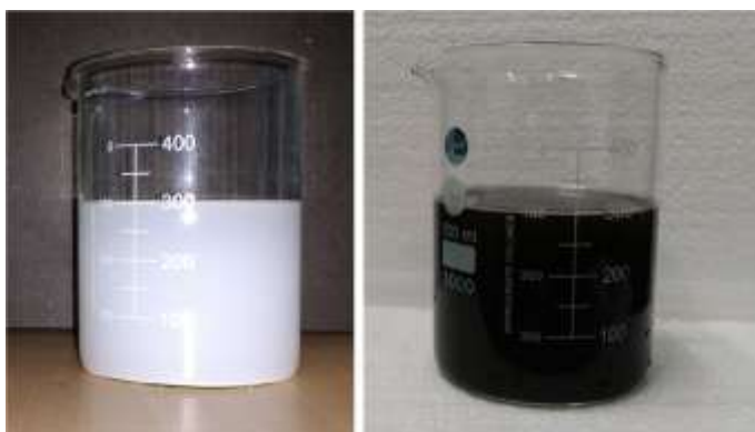
Fig. 3. Al_2O_3 -water and CuO -water nano-fluid (0.05%) [4]
