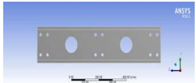
Fig. 5. Lipped channel beams with circular opening.
