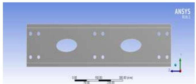
Fig. 6. Lipped channel beams with elliptical opening.
