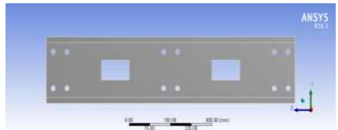
Fig. 4. Lipped channel beams with rectangular opening.
