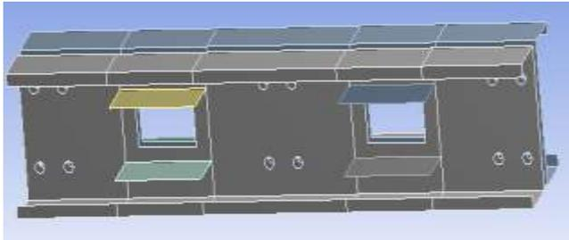
Fig. 8. Rectangular opening with stiffener arrangement 2.
