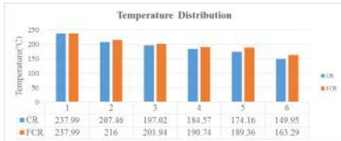
Fig. 4. Comparison for temperature distribution of dome for different concrete mix.
