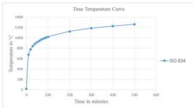
Fig. 2. ISO 834 Time-Temperature curves.
