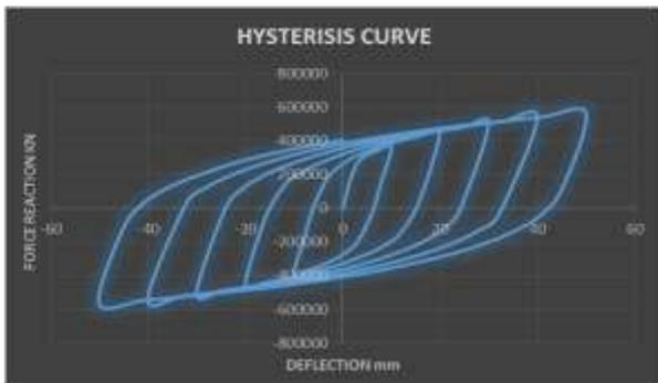
Fig. 4. Hysterisis curve of a typical joint.
