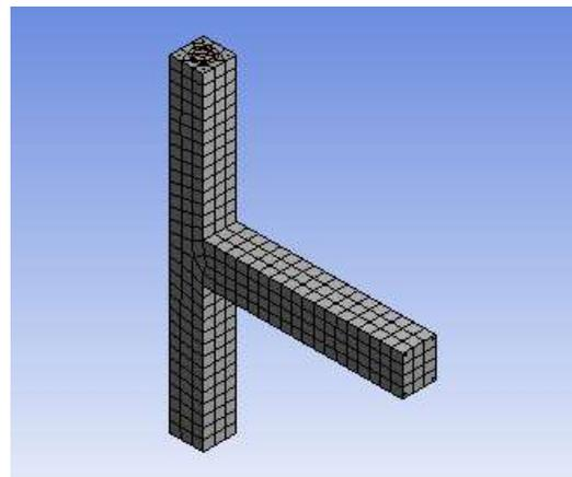
Fig. 3. Meshed view of a joint.
