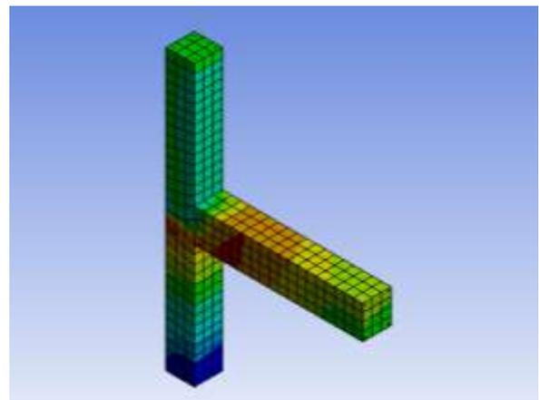
Fig. 3. Total deformation of a typical joint.
