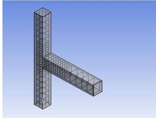
Fig. 2. Model of conventional beam column joint.
