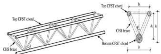
Fig. 1. Schematic view of FEA modelling.
