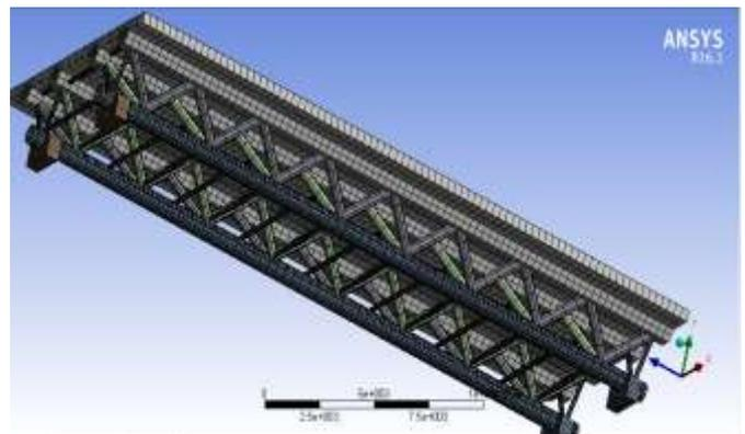
Fig. 6. Meshed view of full scale model.
