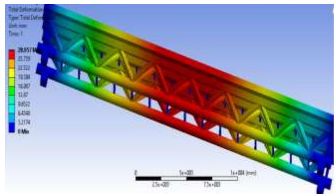
Fig. 7. Deformation of full scale model.
