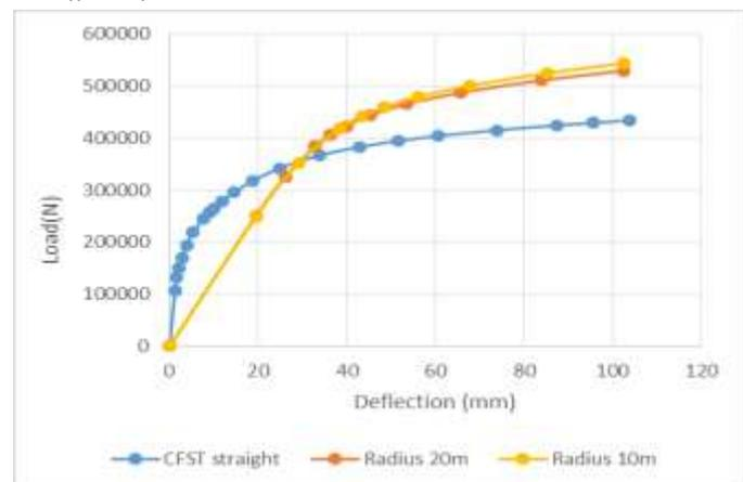
Fig. 4. Straight and curved truss comparison.
