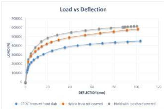
Fig. 5. Effect of concrete slab.
