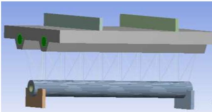
Fig. 2. Perspective view of hybrid CFDST truss.
