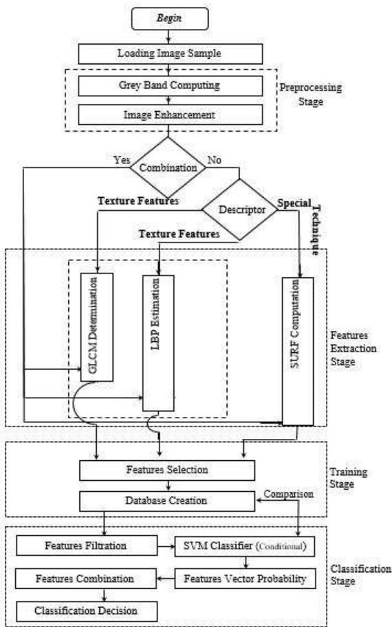
Fig. 2. Block diagram of the proposed satellite image classification.
